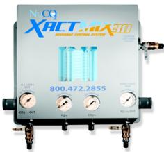
The **XactMix** beverage control system is “command central” for managing beverage carbonation. The system automatically blends and dispenses the precise amounts of beverage-grade carbon dioxide and draft beer-grade nitrogen. It also has a proprietary gas monitoring system that easily identifies even the smallest gas leaks or when the gas supply is nearly empty.
